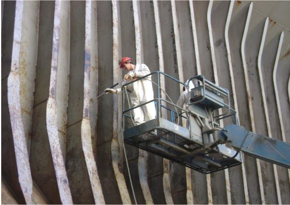
Shore cleaning gang cleaning the Cargo Hold after discharging Cement
