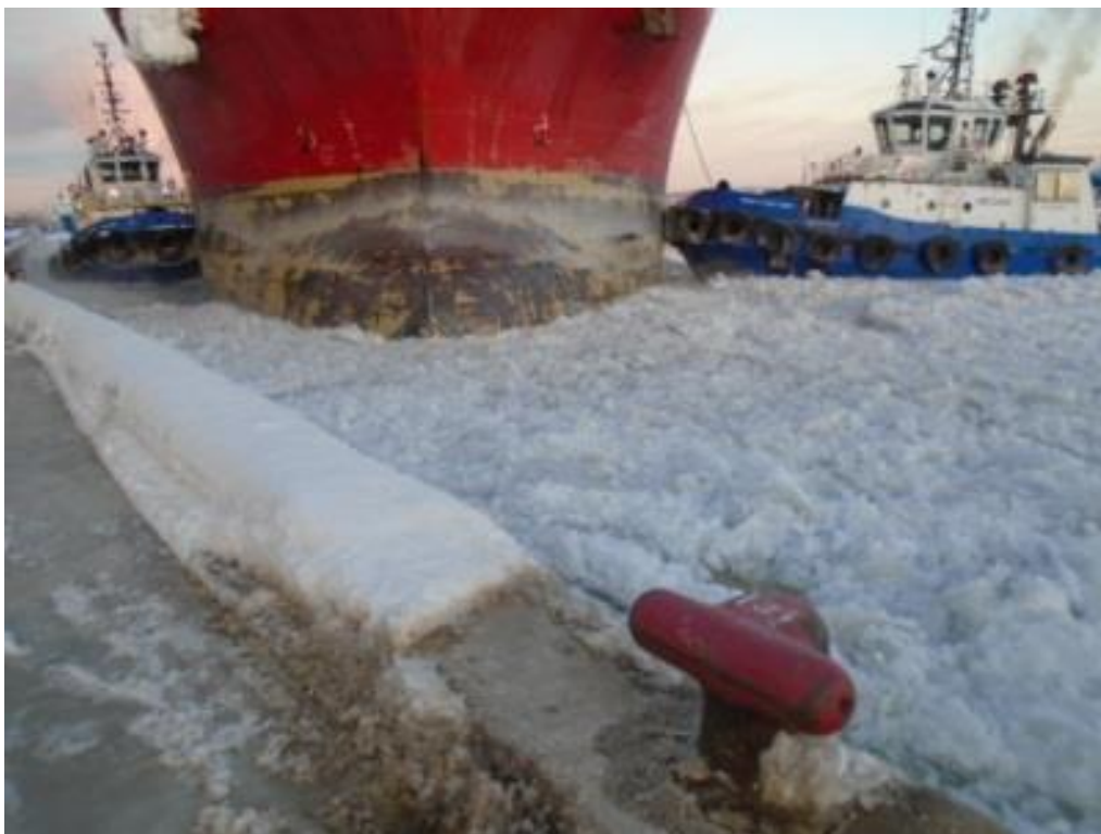
Case Study 2: Vessel approaching berth, tug breaking ice, 2 nd tug pushing
