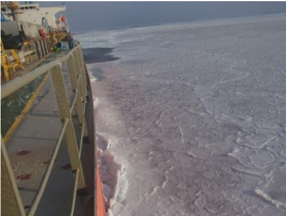
Case Study # 3 Vessel stuck in Ice, accumulation of Ice at Port Side
