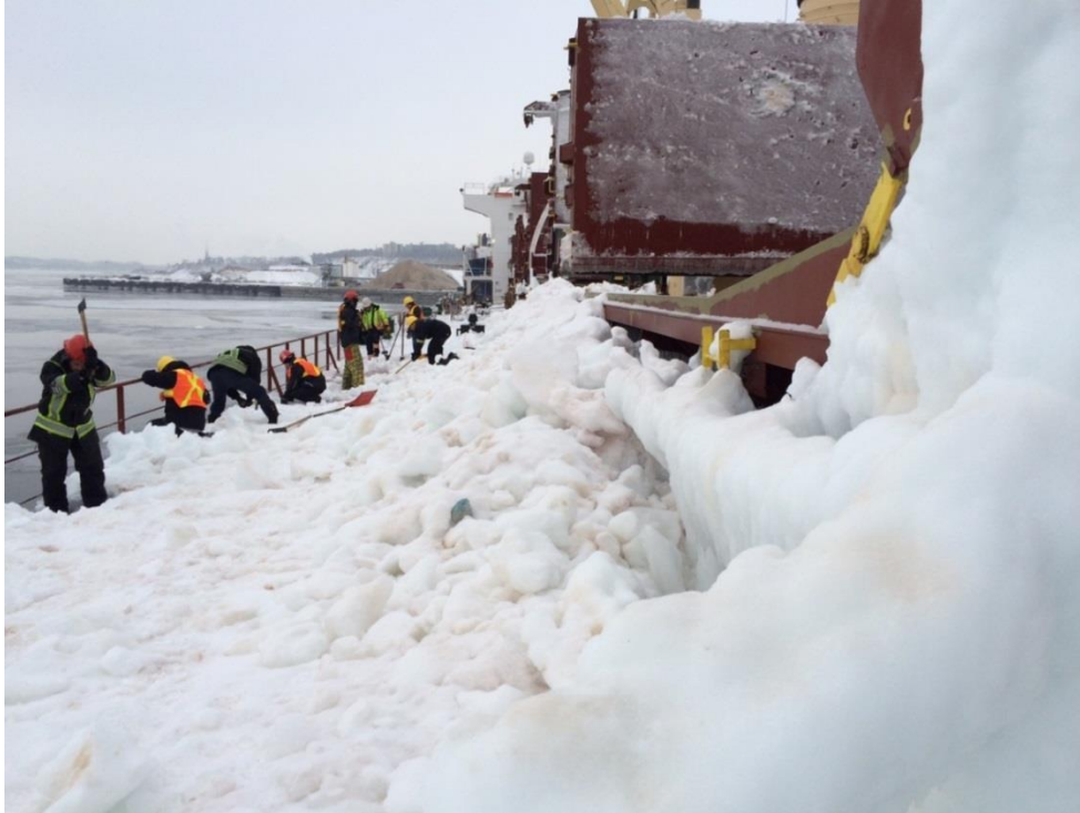
An accumulation about 350 M/T of ice on Deck.
