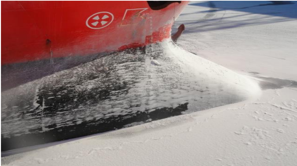
Forward Draft mark, Starboard Side covered with thick 25cm (approximately) ice
